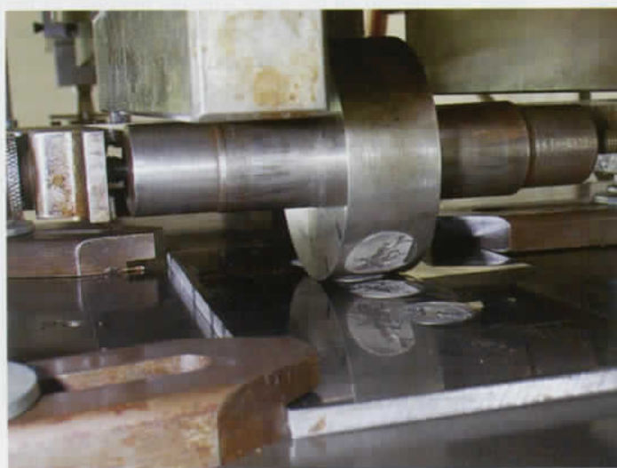
Figure 23. Transfer roll in transfer press with ends of mandrel beneath the bearers which apply the pressure. Courtesy of Michael Bean.
