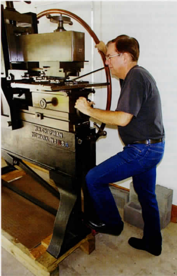
Figure 8. Michael Bean demonstrating a transfer press. The large wheel in his right hand moves the sliding bed forwards and back. The foot lever is pressed to create the pressure between the transfer roll and the plate.
